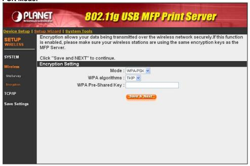
When "WPA-shared key", also named "WPA-PSK" requires users to select the advanced encryption methods, i.e. TKIP and enter a set of shared key.
